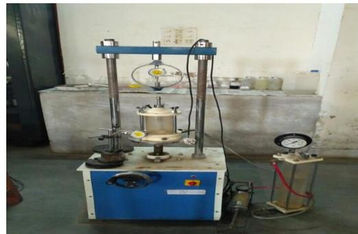
Tri-Axial Test Apparatus
