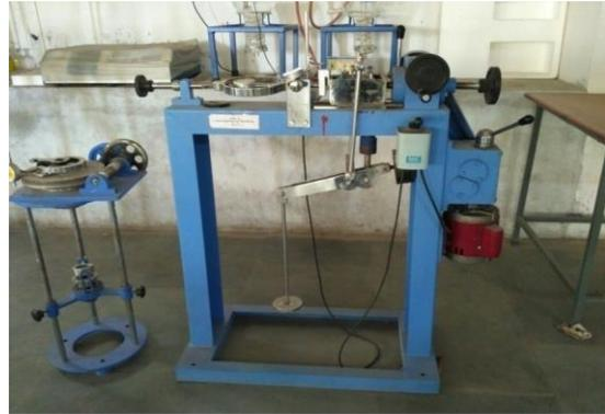
Direct Shear Test Apparatus
