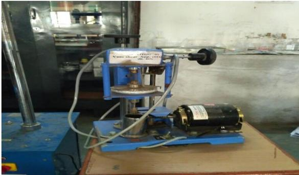
Vane Shear Test
