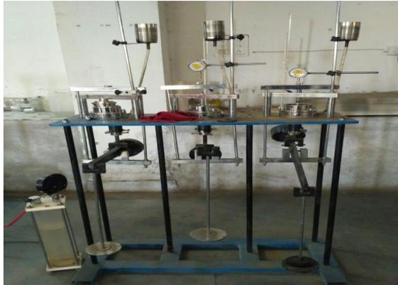
Consolidation Test Apparatus
